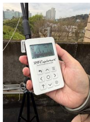
Handheld spectrum For background noise inspection
